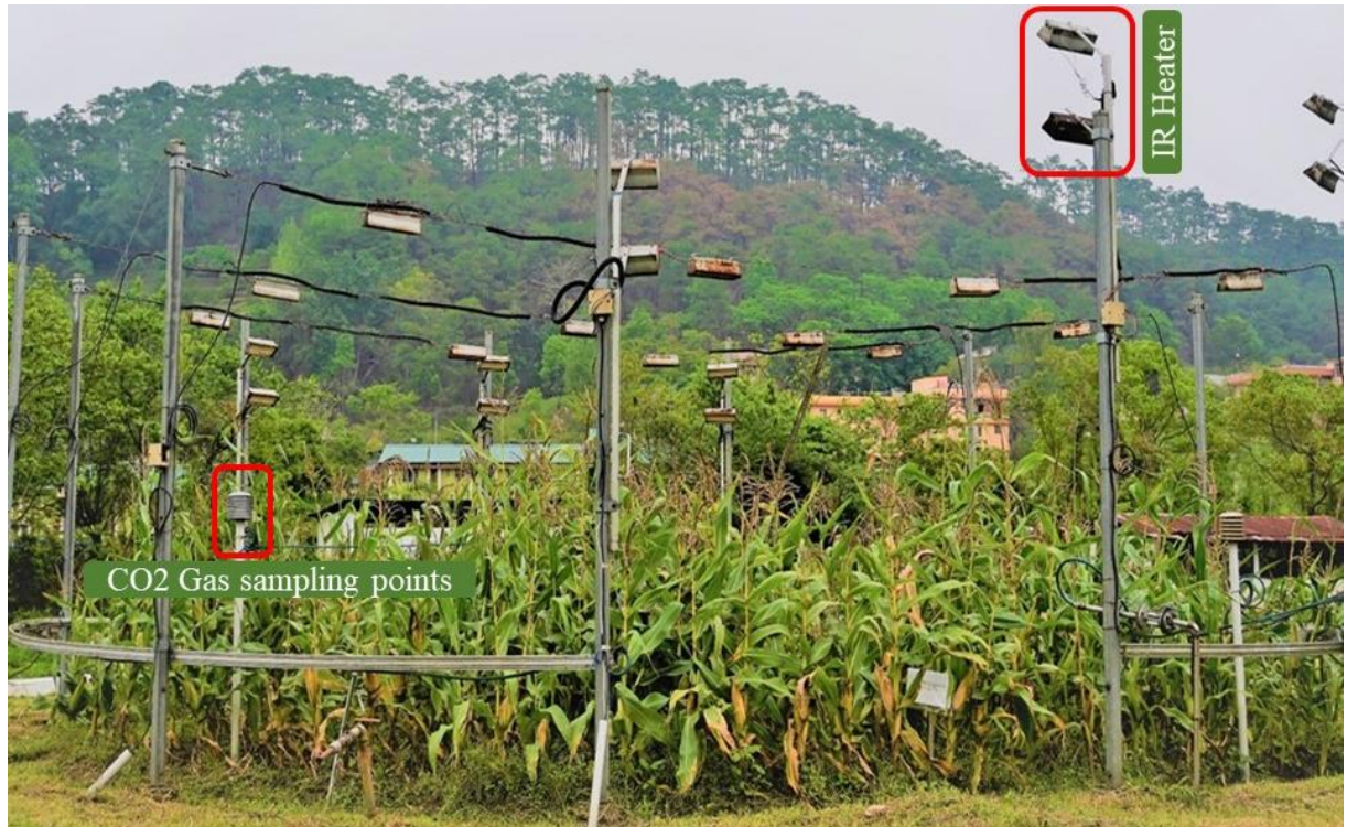
Fig. 10. Elevated CO 2 and elevated temperature rings
