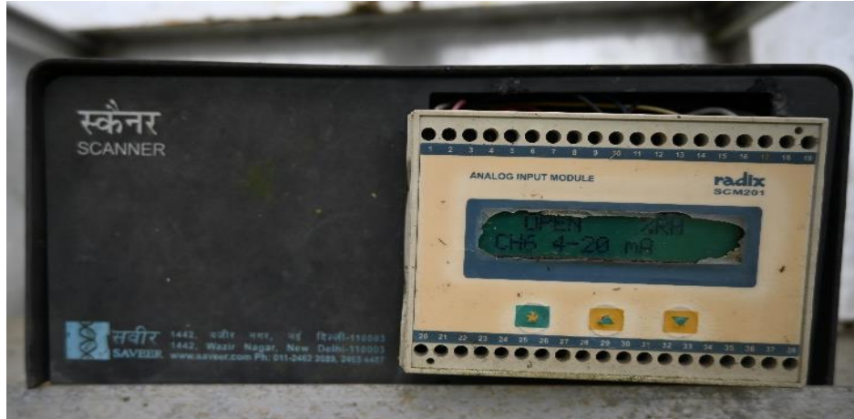
Fig. 13. Analogue Input module- Scanner (Radix- SCM 201)
